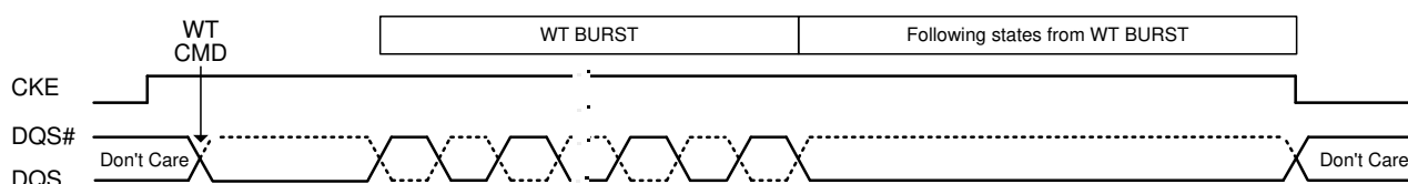
Figure 18. WDQS Control Mode 1 - Read Based Control
