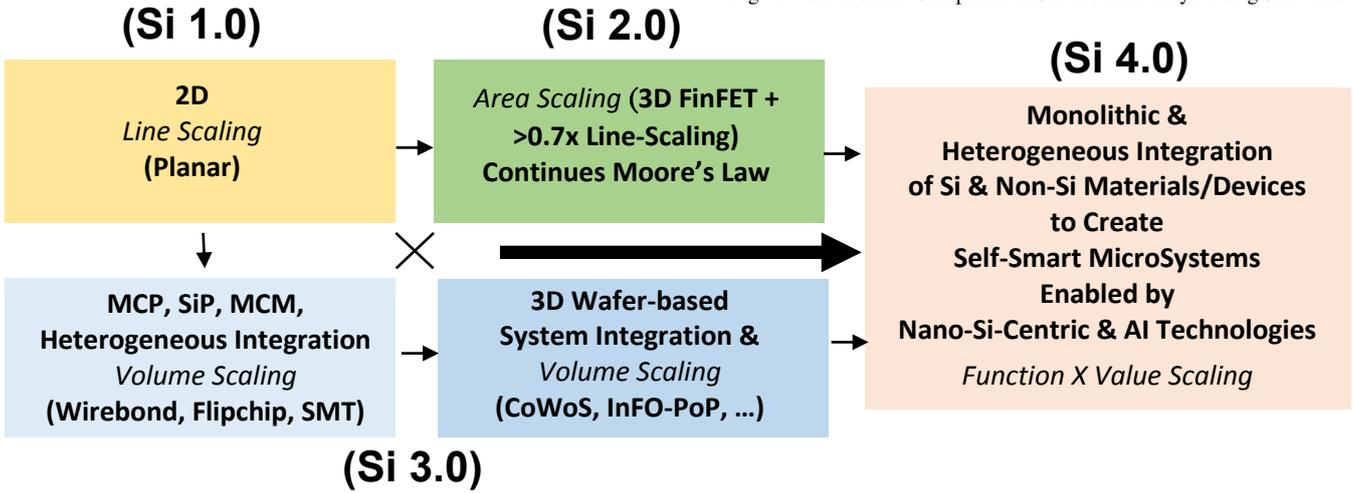
Fig. 2. A Block Diagram Description of Silicon Ages from 1.0 to 4.0 for Past 60 Years.
