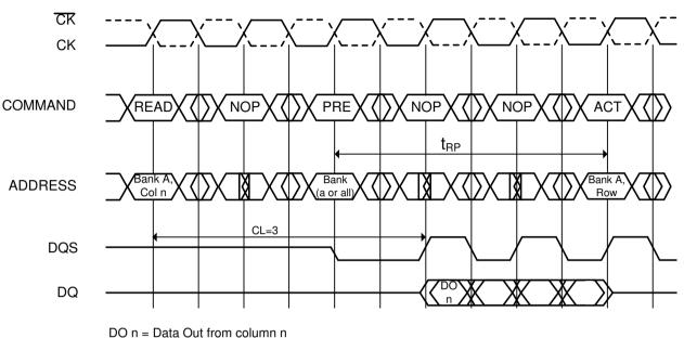
Cases shown are either uninterrupted bursts of 4, or interrupted bursts of 8 3 subsequent elements of Data Out appear in the programmed order following DO n Precharge may be applied at (BL/2) tCK after the READ command Note that Precharge may not be issued before tRAS ns after the ACTIVE command for applicable banks The Active command may be applied if tRC has been met
