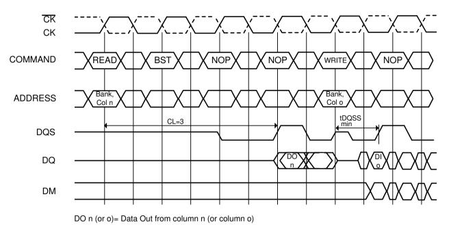
Burst Length= 4 in the cases shown (applies for bursts of 8 as well; if burst length is 2, the BST command shown can be NOP)
