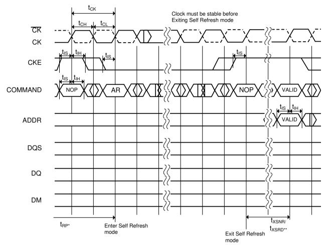
\* = Device must be in the "All banks idle" state prior to entering Self Refresh mode \*\* = tXSNR is required before any non-READ command can be applied, and tXSRD (200 cycles of CK) is required before a READ command can be applied.
