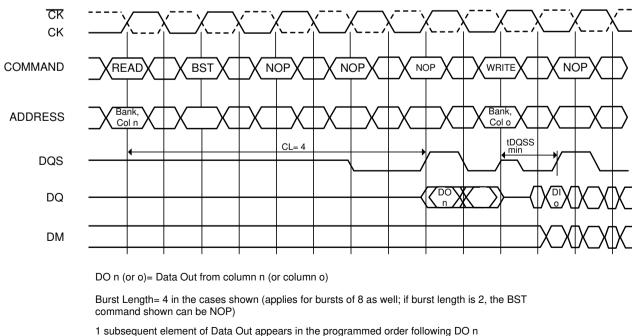
Figure 32. Read to Write Required CAS Latencies (CL=4)
