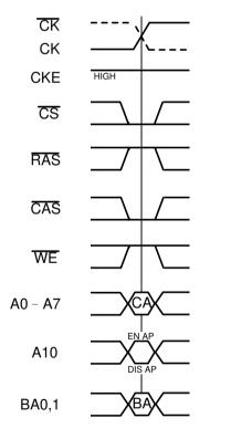
CA=Column Address BA=Bank Address EN AP=Enable Autoprecharge DIS AP=Disable Autoprecharge
