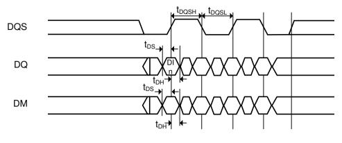
DI n = Data In for column n Burst Length = 4 in the case shown 3 subsequent elements of Data In are applied in the programmed order following DI n
