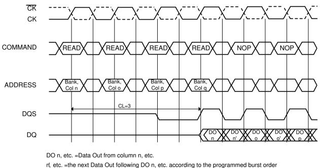
Burst Length=2,4 or 8 in cases shown. If burst of 4 or 8, the burst is interrupted
