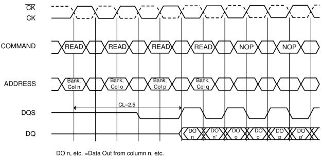
rl, etc. =the next Data Out following DO n, etc. according to the programmed burst order Burst Length=2,4 or 8 in cases shown. If burst of 4 or 8, the burst is interrupted Reads are to active rows in any banks
