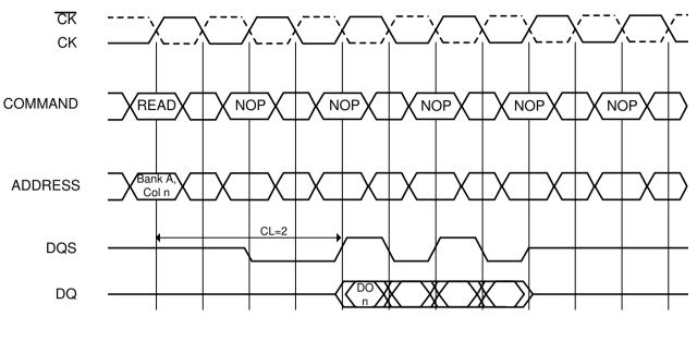
DO n=Data Out from column n Burst Length=4 3 subsequent elements of Data Out appear in the programmed order following DO n
