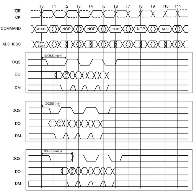
DI n = Data In for column n 3 subsequent elements of Data are applied in the programmed order following DI n A non-interrupted burst of 4 is shown A10 is LOW with the WRITE command (AUTO PRECHARGE disabled) DM=UDM & LDM
