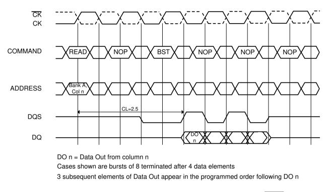
Figure 27. Terminating a Read Burst Required CAS Latencies (CL=3)
